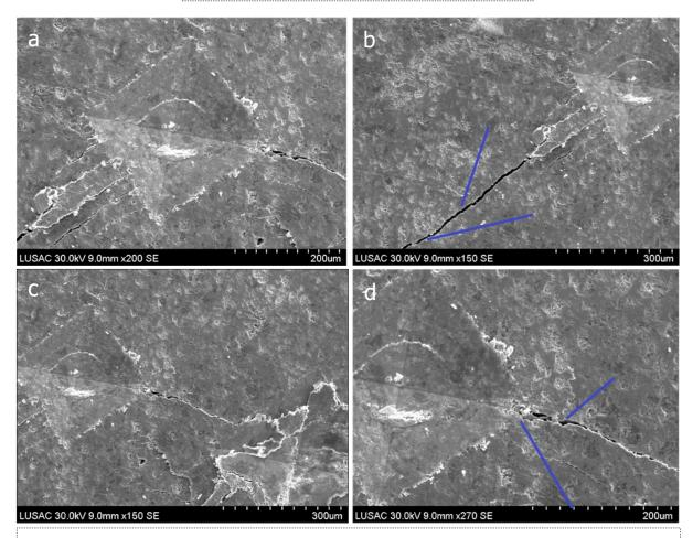
Figure 7. SEM, BSE micrograph of cracks at the corners of Vickers indents: of etched MTC showing a purely transgranular crack growth; and revealing an intergranular crack with deflection and crack bridging: (a)-Transgranular crack, (b)- Intergranular crack, (c)- Crack deflection, d- Crack bridging
