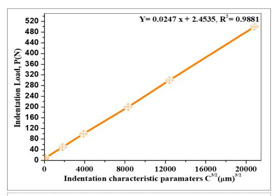
Figure 9. Correlation in between the applied load P, and half-length of median crack  $c^{3/2}$  of MTC polished and etched surface for the sintered samples using a 20 mm diameter die
