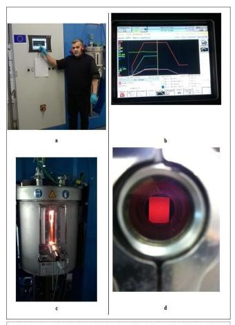
Figure 1. SINTER-LAB, FCT-HP D 25, SPS-1050, ENSICAEN. (a)-The author, (b)-Variation of the displacement, the displacement rate and the temperature in dependence of the heating time, (c, d)- The plasma produced by the current in the SPS chamber.
