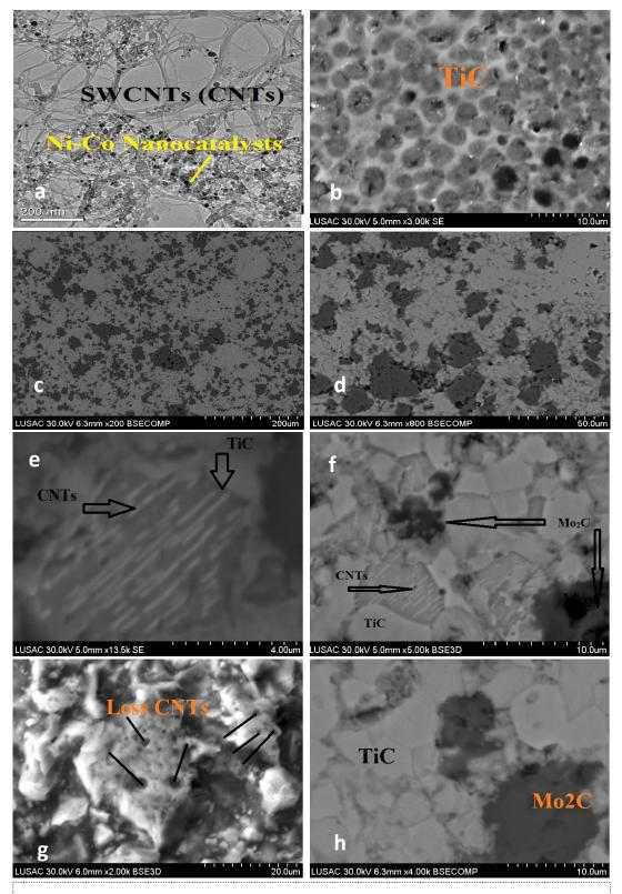
Figure 3. High magnification microstructural representative SEM image of MTC polished and etched surface for the sintered samples using a 20-mm diameter die. (a)-TEM of SWCNTs, (b)-SinteredTiC grains , (c)-Nanocompositesoverview, (d)- nanocomposites overview with magnification, (e)-SWCNTs into the TiC grain, (f)-SWCNTs into the TiC grains ,(g)-Pore like structure of losses SWCNTs , (h)-Nanocomposites overview with higher magnification.
