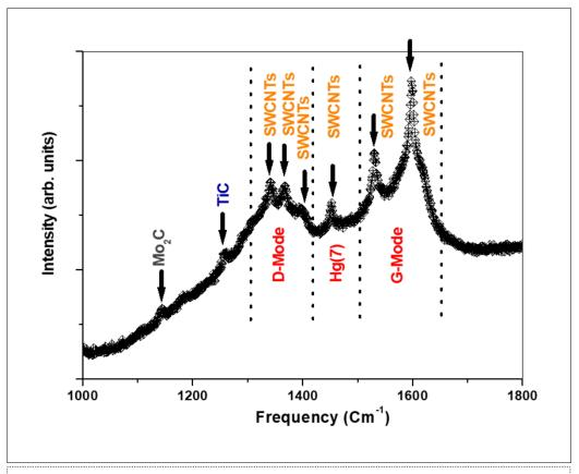
Figure 10. Raman spectra of the synthetized samples using a 20 mm diameter die.
