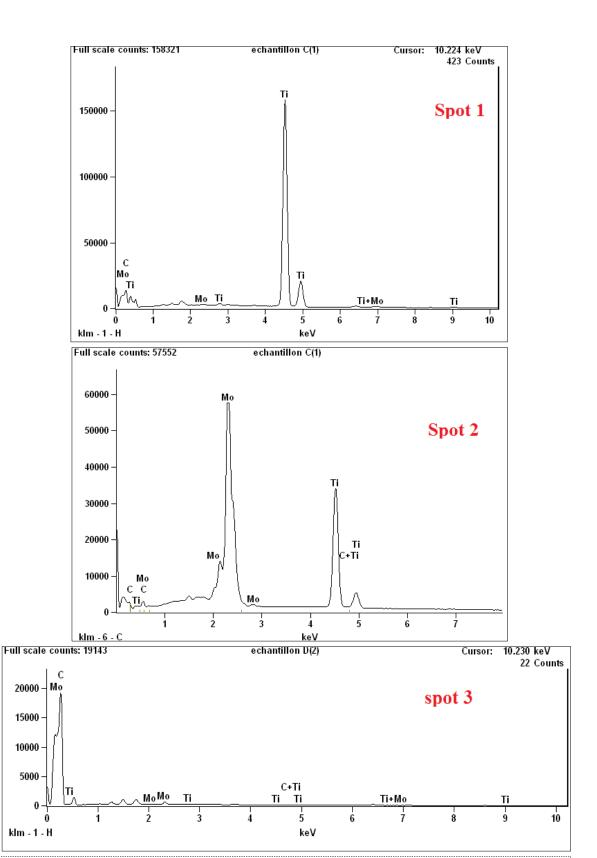
Figure 5. EDX spectra in different regions of MTC polished and etched surface for the sintered samples using a 20-mm diameter die:  $(Spot_1)$ - TiC regions,  $(Spot_2)$ -Mo<sub>2</sub>C regions,  $(Spot_3)$ -SWCNTs regions
