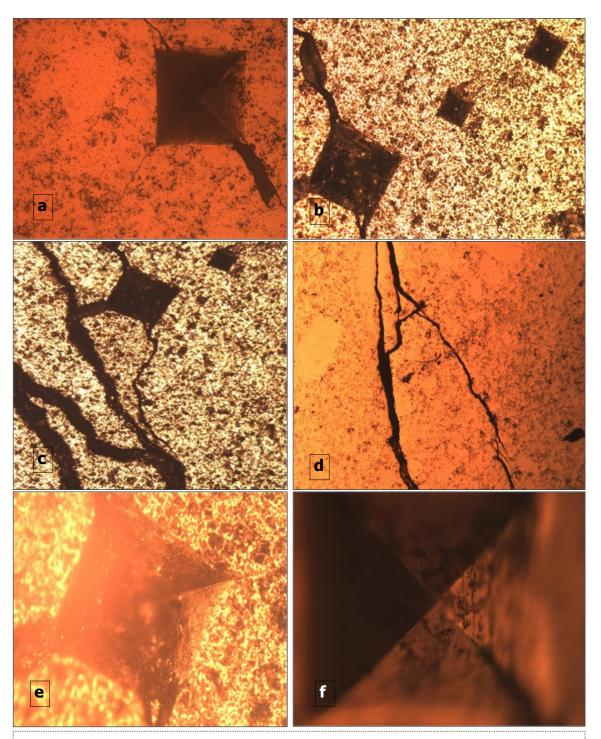
Figure 8. Optical micrograph of crack patterns used for IFT calculations of (a, b)-MTC tested at 300 N, (c)-MTC tested at 500 N. Micrographs of cracks at the corners of Vickers indentation: (d)-Etched MTC showing a purely transgranular crack growth and (e, f)-High magnification of indentation label.
